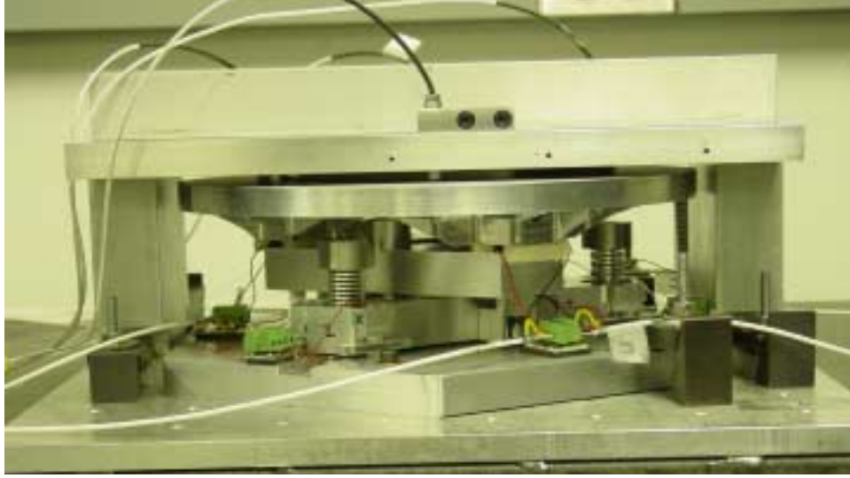
Figure 18: Fast steering mechanism and metrology fixture
