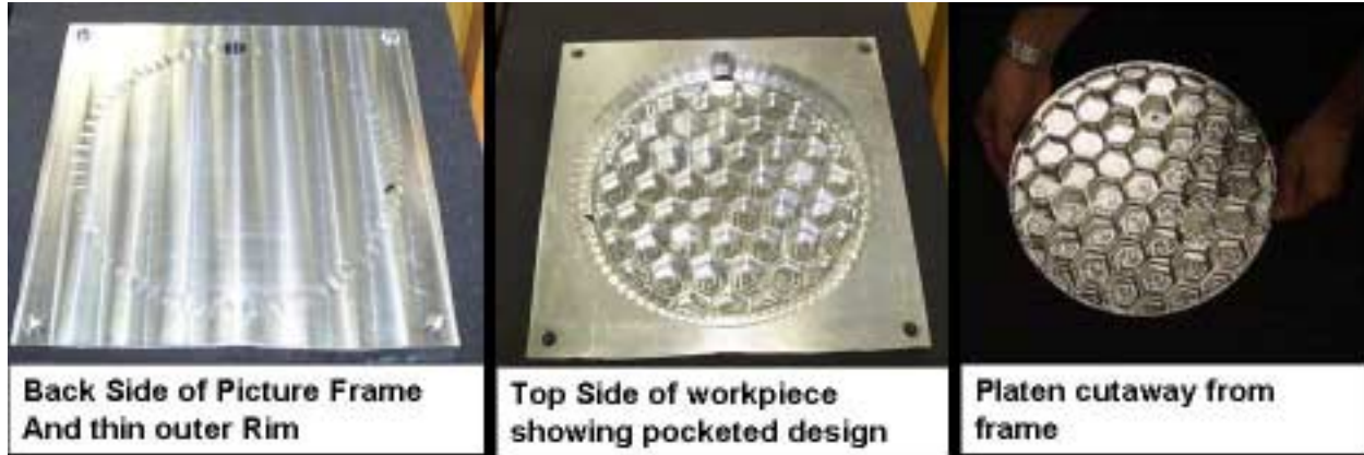
Figure 7. Manufactured platen representing the 300 mm mirror (manufactured in 2.5 hours).
