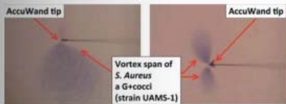
Figure 4 Rapid sample collection. Vortexing violet-stained S. aureus (strain UAMS-1), attracted in 30 sec at a concentration of 10^4 per mL.
