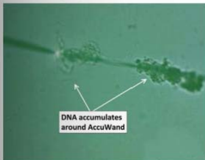
Figure 5 DNA collects on the fiber 180 sec total in liquid and DNA concentrates more.
